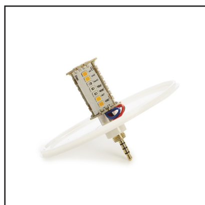
Phase 3: to get to the jack led, remove = pull off/pop-off the head from the diffuser
